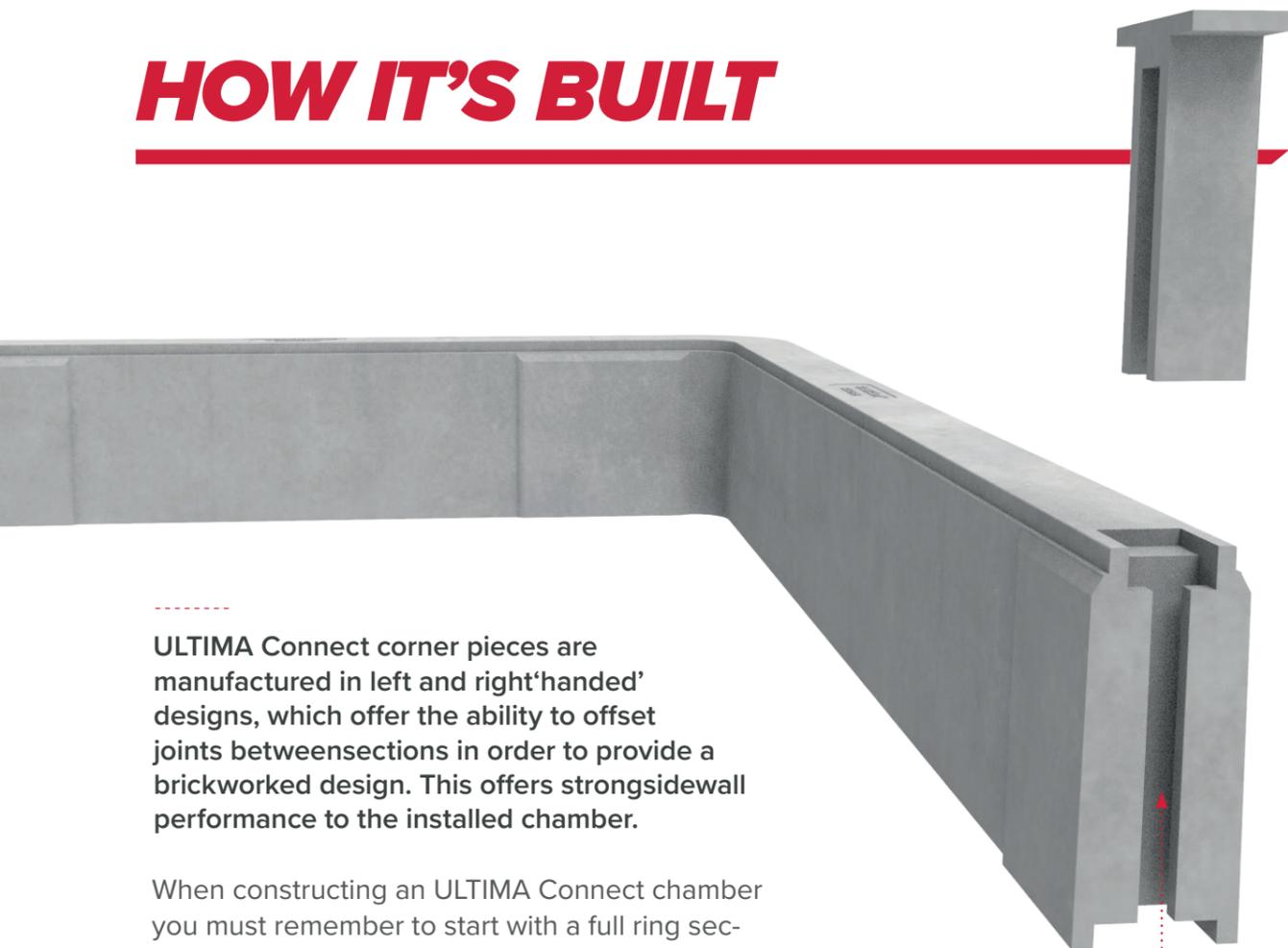
ULTIMA Connect corner pieces are manufactured in left and right 'handed' designs, which offer the ability to offset joints between sections in order to provide a brickwork design. This offers strong sidewall performance to the installed chamber.
