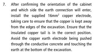
Ensure the copper electrode is run for the full length of the duct trench (ideally for 2m). If this is not
