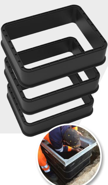
Built by stacking ring sections to the required depth, each Modula part weighs under 11kg, making the suitable for a single person lift under manual handling regulations. X-TRAS™ cable management, MULTIduct™ Spigots and duct entries provide a complete chamber systems solution for a range of sector applications.
