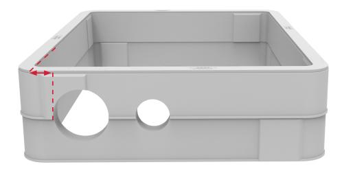
When drilling two duct entries side by side, a space half the diameter of the larger duct must be left between them.
